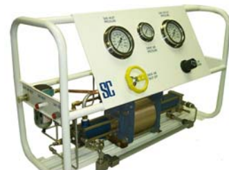
GBD & GBT Series Double Acting Booster 5:1 thru 150:1 Ratio Single & Double Head Pressure to 25,000 psi
